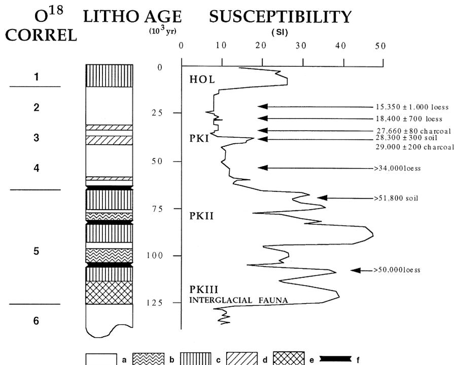
Fig. 5. Loess sequence in Vestonice (Czech Republic). Variation of magnetic susceptibility, lithology and  $^{14}\text{C}$  dates (Klima et al., 1962) Plotted on the age scale. Lithology: (a) loess, (b) pellet sands, (c) chernosem, (d) arctic brownearth (e) B-horizon of a forest parabraunerde, (f) marker. PKI–II: numbered pedocomplexes. In the left margin correlation with marine isotope stages.
