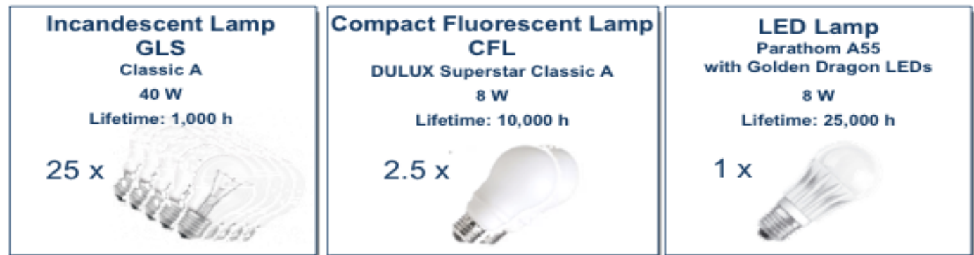
Figure 2: Type of lamps compared in the Life Cycle Assessment: a 40 W incandescent lamp, a compact fluorescent DULUX Superstar and a Parathom LED lamp output between 345 to 420 lm
